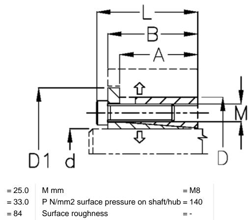
D1 mm = 45 d H8 mm = 75 D mm Fit tolerance = -F kN torque = 80 L mm = 41
